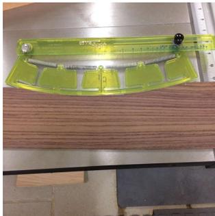
The bevel block can be made of a soft, light wood, that is easy to shape. I used a block of western red cedar I had. Basswood is fine too. You end up with a banana type shape by the time you are through that transitions smoothly back to your kerfing.
