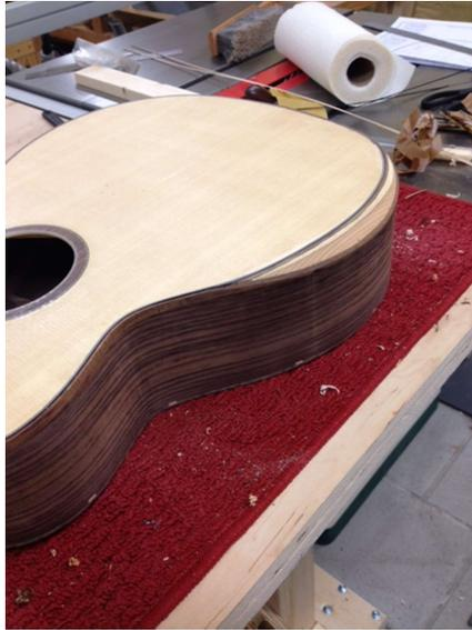
I smoothed the bevel flat along the curve using a block plane and finished off with a scraper and finally with a sanding block. This doesn't take very long. Try to leave as much material on the binding pieces along the top and bottom as possible. It gives you more of a safety net for your veneer later.
