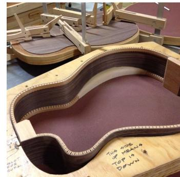
Note the ledge between the bevel block and the side in the center picture. This will hold the binding you will place on it later.
