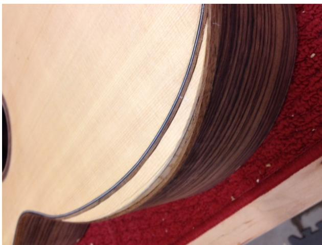
Notice how the piece of top cutoff material that is shaped to fit in after the purfling and binding piece on the top. *I told you it would be used later.*
