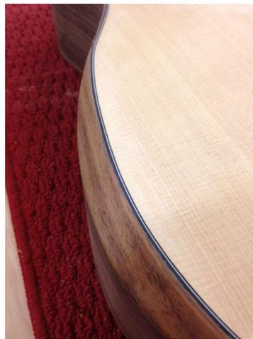
Pictures above show gluing and taping of veneer and finished bevel. Notice how the veneer blends into the bindings on both the top edge and side edge.
