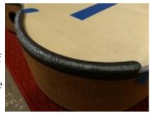
Below is the armrest in its final shape and form before installing. I still have to do final prep work on the guitar before finishing. I will tape off the guitar top at the area to allow for the armrest. The armrest will be glued on after the bridge, as one of the last items to complete the guitar.
