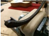
The material on the inner face is removed, again, using my spindle sander. I sand the edges as uniform and consistent as possible. This will make any final sanding by hand easier as I soften those edges. In this picture note the lower section that will glue to the top. It does not exceed the width of the lining beneath the soundboard. This allows for the full soundboard to vibrate as originally designed.
