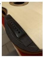
I now determine how wide I want my armrest to be. Using the outer contour, I place a ruler and mark off 12mm ( $\sim 1/2$ ") along the curve to give it a uniform width for this particular design. Remember "Your guitar, Your rules!" You have flexibility in your design. Being that this is mostly refining of the shape, I use my spindle sander.
